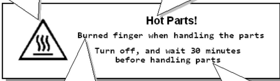
**Element 3**: Text that describes the possible consequences of energy transfer from the energy source to a body part.
