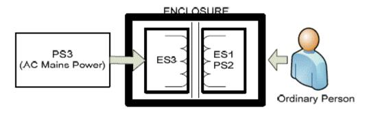
**Example 2: Non Accessible Solid Safeguard** - In this example, the internal metal shield serves as an *electrical enclosure* (non-accessible solid safeguard) and a separate external plastic enclosure serves as a *fire enclosure* (accessible). Only the *fire enclosure* is evaluated for robustness as it is the accessible safeguard.
